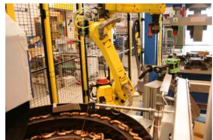
<< Vision Guided Robot picks up fittings from a bowl feeder and loads them into a free issue press
