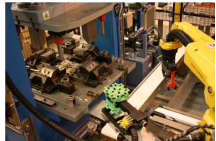
<< Vision Guided Robot picks up fittings from a bowl feeder and loads them into a free issue press
